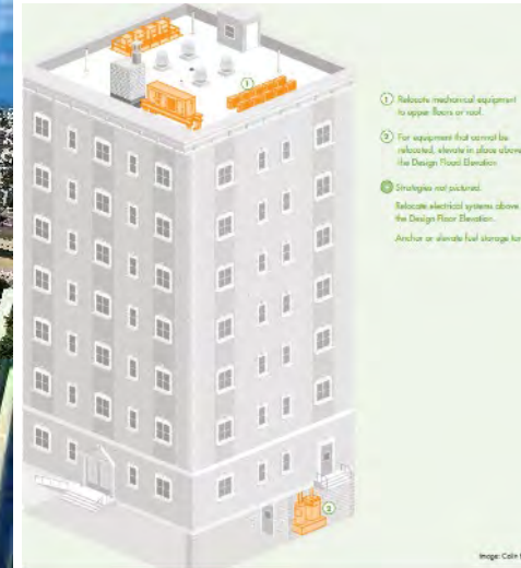
Relocated Mechanical Equipment
